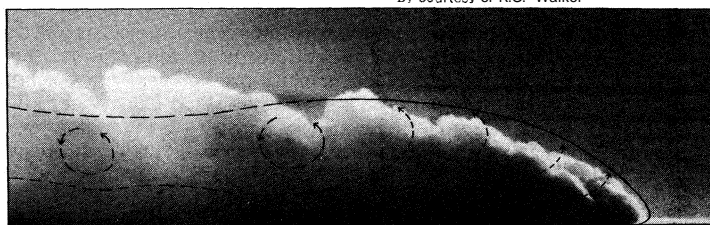
Figure 3: Motion within the head of an experimental density current, showing characteristic shape of head, upward diverging flow, breaking away of eddies from the back of the head. Depth of water is about 30 centimetres.
